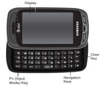
Your a877 has a built-in, keyboard-style keypad, commonly called QWERTY, that you can access by sliding it open from beneath the top section of the phone. This also automatically rotates the image in the display to show information in a wider, landscape format. Using the QWERTY keypad, you can type letters, numbers, punctuation, and other special characters into text entry fields or other applications simpler and faster than using the telephone keypad.
